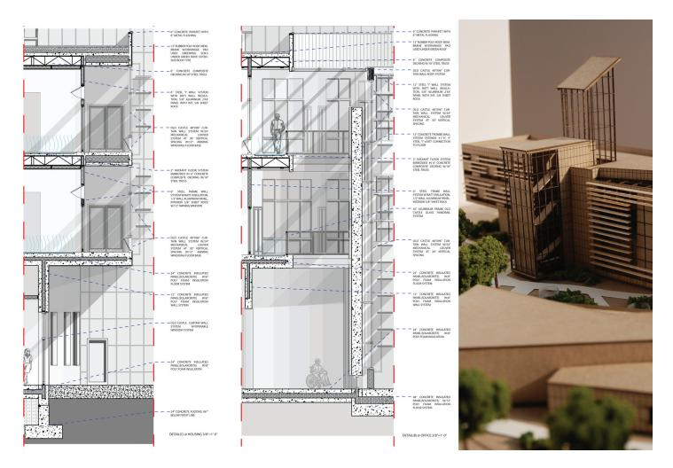
Figure 5. The building envelope as thermal capturing device (Xuefeng Zhong, Gregory Uhrich, Tim Lewis).
