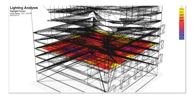
Figure 1. Daylight analysis for one floor level in Rhinoceros / Autodesk Ecotect to understand how a 3 dimensionally distorted courtyard enriches the daylight uniformity of internal spaces (Suncica Jasarovic, ARCH 490, Spring 2012).
